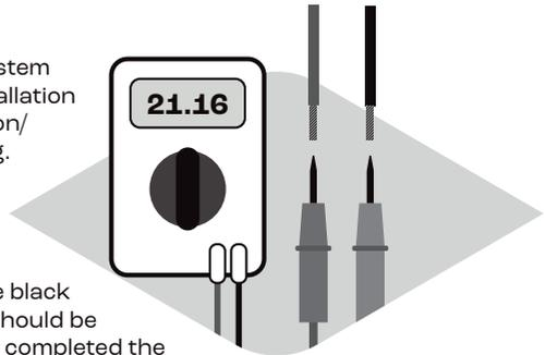
There is the possibility of a degree of variance in the readings that you take during the course of the installation. If this is not too significant (5% either way) you should not worry too much as the reading can be affected by moisture and other factors. We recommend that you test the floor sensor with an ohm reading (generally 8 to 20 ohms). The sensor is covered by the thermostat guarantee (usually between 3-5 years).
