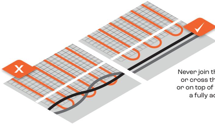
Never join the heating element wires or cross the cold leads underneath or on top of the mats. Our mats have a fully adhesive sticky backing to stick to the sub-floor.
